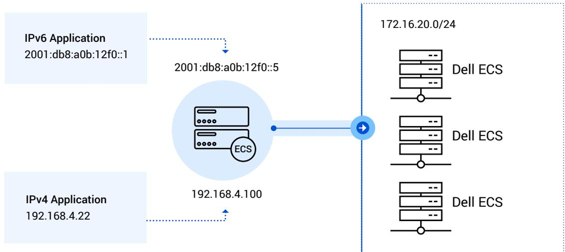
In the example above, the IPv6 and IPv4 applications have concurrent access to ECS with the ECS Connection Manager providing network isolation. Multiple IPv6 and IPv4 networks may be supported with options to isolate using VLANs or with physically different network ports on hardware appliances.
