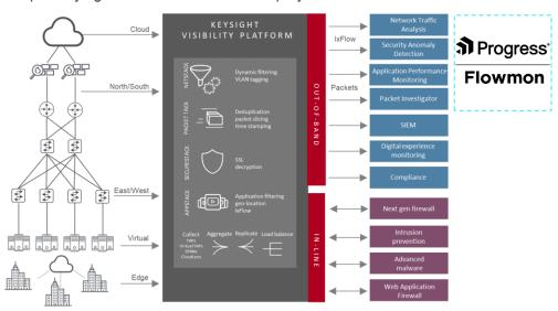
How it works: Keysight visibility solutions provide packet or enhanced netflow data from physical, virtual, and cloud access points to Flowmon, simultaneously aggregating, filtering, and directing exactly the right data to each tool.
